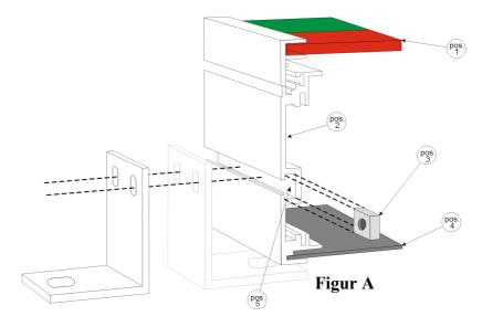
supports it while the mountings are fastened to the square nuts by the enclosed bolts (*Appendix I* - *figure 3*) and washers (*Appendix I* - *figure 4*).
